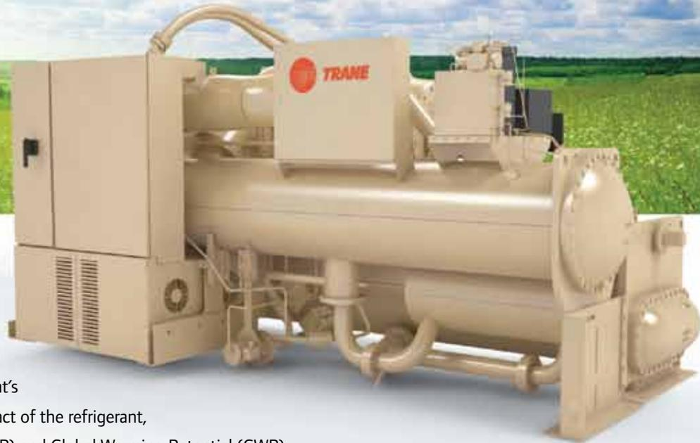
Direct-drive CenTraVac™ chillers are designed to use a low-pressure refrigerant. This means the chillers operate in a vacuum, which virtually eliminates leaks and enables near-zero emissions throughout their operational life. That's a win in terms of the direct environmental impact of the refrigerant, minimizing the Ozone Depletion Potential (ODP) and Global Warming Potential (GWP).
